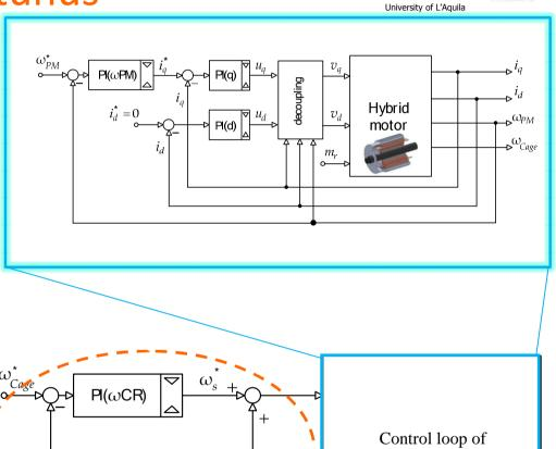
The outer control loop compares the imposed cage-rotor speed with the actual value calculated by Flux.
