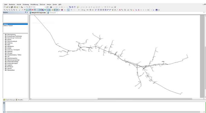
The GIS import interface supports common exchange formats (Shape, Stanet) and offers a high degree of flexibility due to its extensive configurability. In addition to the information held in the GIS, other data sources can be included in the import.
